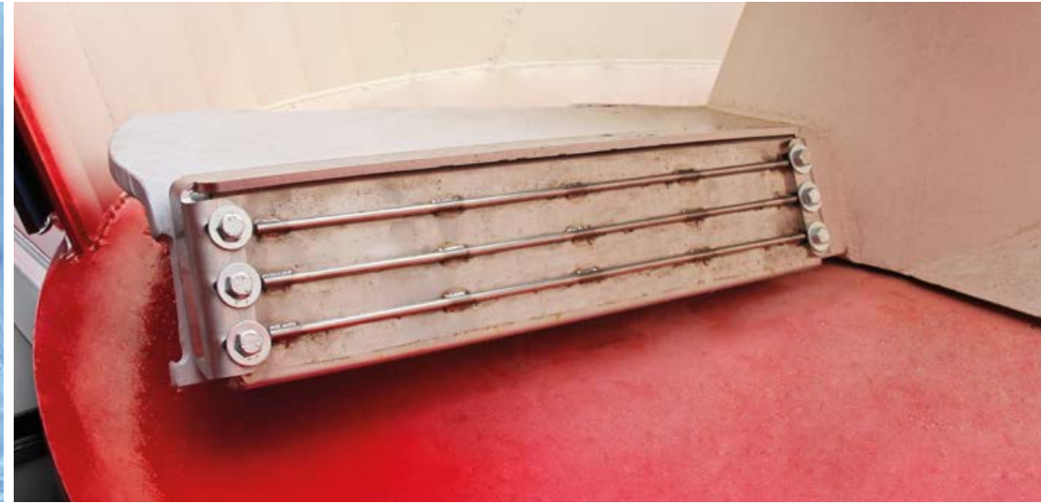
Heavy-duty magnet on the turbo auger.
