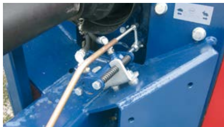
Hydraulic shift for 2-speed gearbox.
