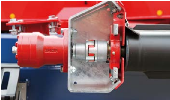
The coupling between the drive motor and the drive roller provides for straight running and long service life.
