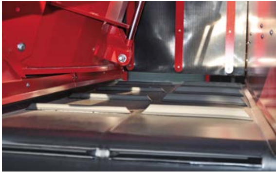
The SILOKING Cross conveyor belt works with slats of different heights for higher performance and more operational reliability.
