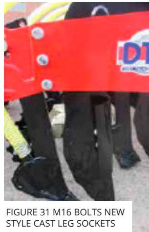
FIGURE 31 M16 BOLTS NEW STYLE CAST LEG SOCKETS
