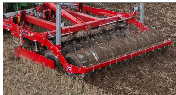
FIGURE 6 CREATION OF A SHALLOW STALE SEEDBED
