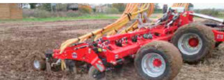
FIGURE 23 ENSURE SEEDER UNIT IS PRESSURISED INTO WORK POSITION
