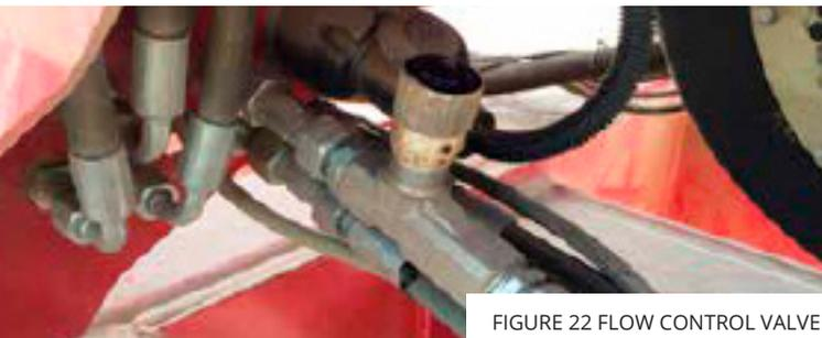
FIGURE 22 FLOW CONTROL VALVE
