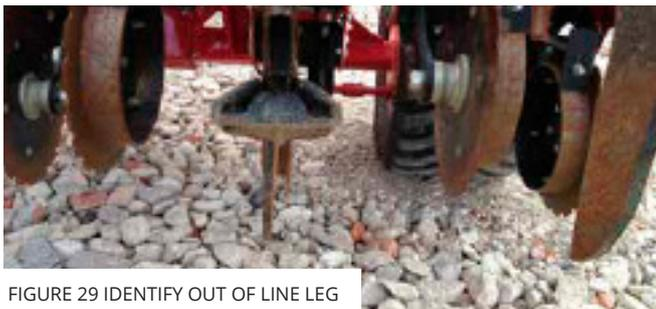
FIGURE 29 IDENTIFY OUT OF LINE LEG
