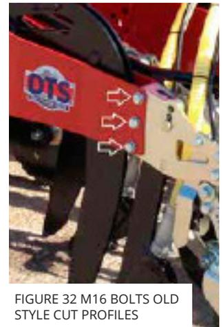
FIGURE 32 M16 BOLTS OLD STYLE CUT PROFILES
