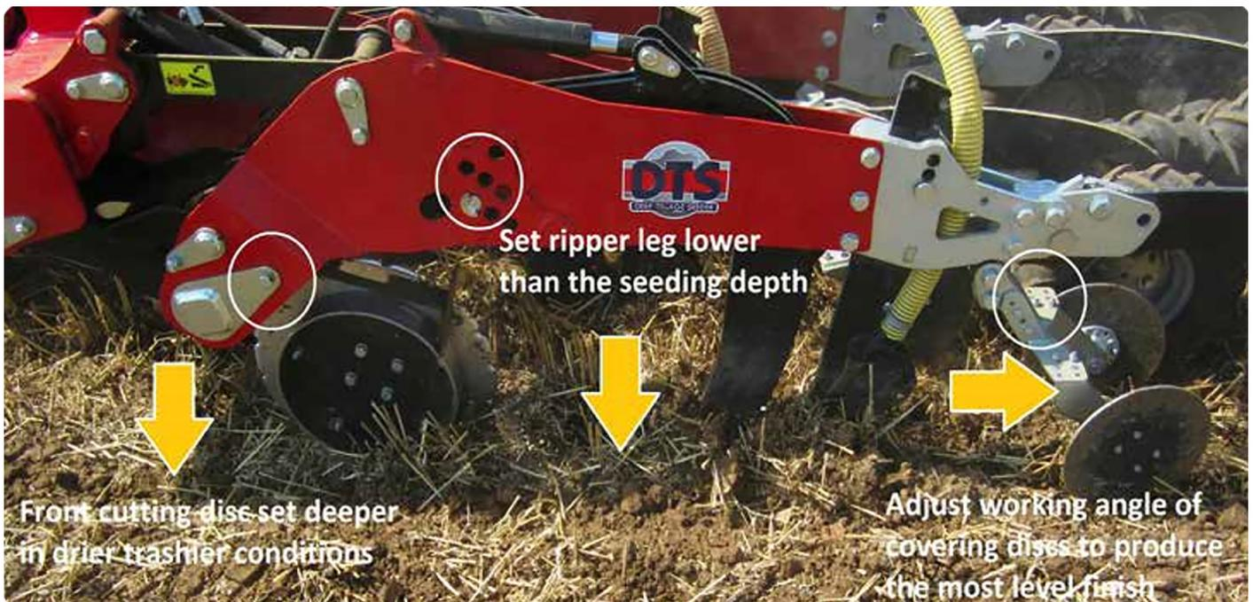
FIGURE 28 MOST EFFECTIVE DTS COULTER SETUP
