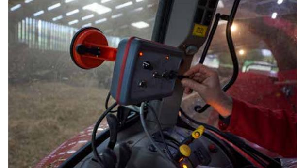
The 4-stage swivel chute is operated by the intuitive controlbox joystick.
