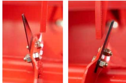
A Kverneland patented system - the knives pass the fixed comb on alternative sides for a more even cut.
