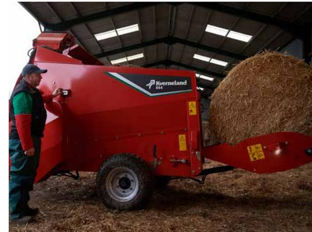
Operating both tailgate and floor chain in safe distance from the moving parts, by using the remote control placed on the side of chamber.
