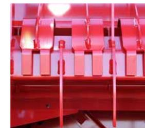
DFCS disengaged for maximum flow through the flywheel.
