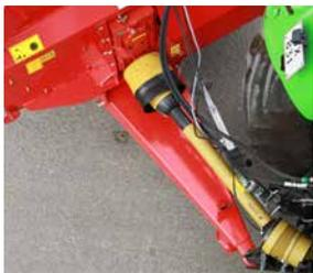
Long drawbar and wide angle PTO for improved turning with larger tyred tractors is standard.
