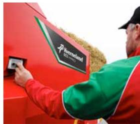
Operating both tailgate as well as floor chain in a safe distance from the moving parts by using the remote control placed on the side of the 853 Pro.
