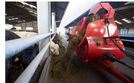
The hydraulically driven swivel chute operates in 4 stages which optimises the blowing distance when bedding.
