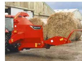
The special design of the tailgate and optional bale retainer offers the possibility to carry an extra round bale.
