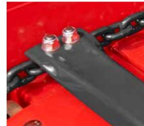
The conveyor slats are designed for **quick and easy individual replacement**.
