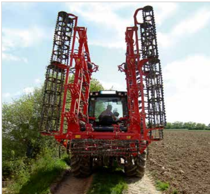
Both, TLD and TLG have three-section foldable frame, which ensures a transport with less than 3.00m.
