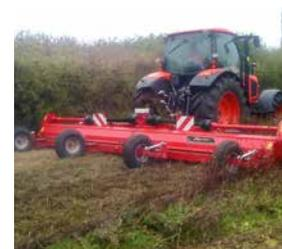
Semi pivoting wheels (10/8.0 x 12.8 ply) available as option ensure good stability and a constant working depth during field operation.
