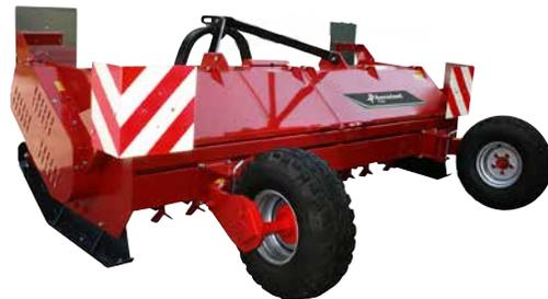
Semi pivoting wheels (10/8.0 x 12.8 ply) as standard ensure good stability and a constant working depth of the FXZ during field operations.
