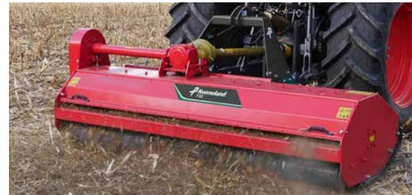
FXE can be equipped with a rear roller (195mm diameter) or 2 semi-pivoting wheels (155 SR13) for a constant control of the working height.
