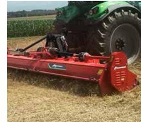
The central gearbox (250hp) is equipped with free wheels; the lateral transmission with automatic belt tensioners ensures reliability and a low maintenance requirement.
