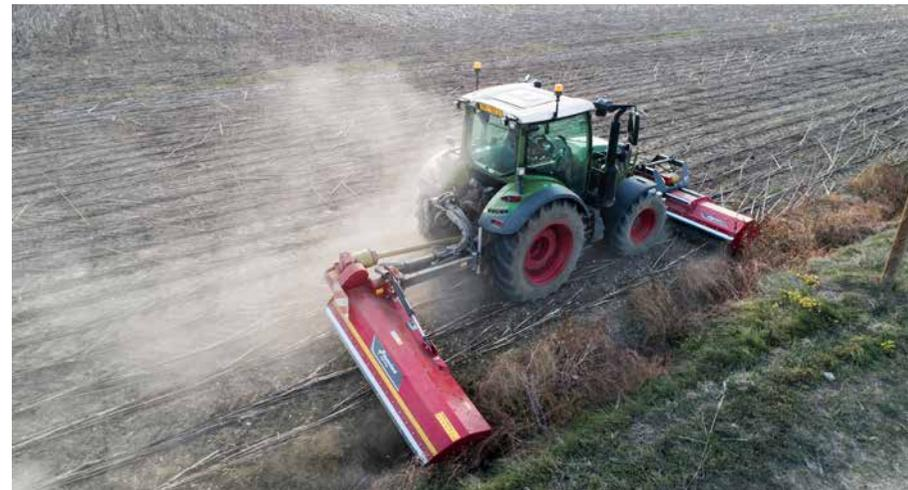
Robust and guarded. Main frame and parallelogram articulations designed according FEM analysis and calculations; heavily tested in Kverneland Klepp laboratory to ensure reliable and long working life. Gearbox and transmission protected against misuse during operation.
