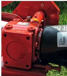
All gearboxes on Kverneland choppers range feature as standard an integrated free wheel.
