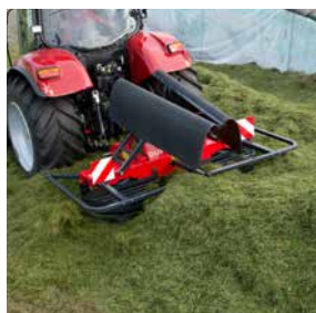
The silage spreader can be operated with either side boards up or down.
