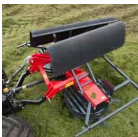
Silodisk can be used as front or rear mounted machine.
