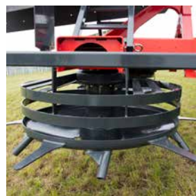
Two drums with aggressive vertical pipes ensure efficient spreading of the crop.
