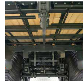
Chain-and-slat conveyor with split driveline and gearbox positioned in the middle.
