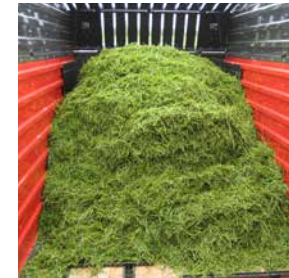
Strong and straight side walls ensure smooth transfer of crop to the rear of the chamber.
