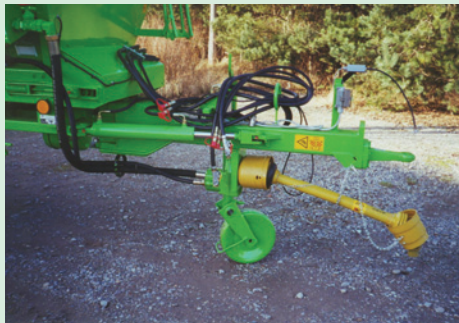
Electro-hydraulic steering drawbar.
