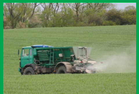
Mounted spreader on converted lorry.
