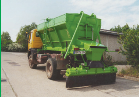
Mounted spreader for soil stabilisation.
