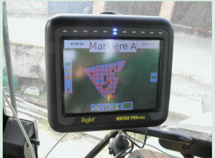
Partial areas specific spreading with „Matrix Pro“.
