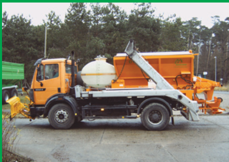
Mounted gritter for spreading moistly salt (winter road services).
