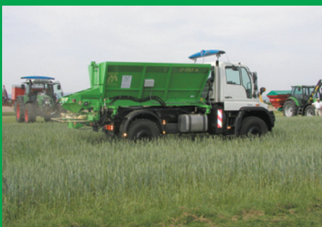
Mounted spreader on MB - Unimog.
