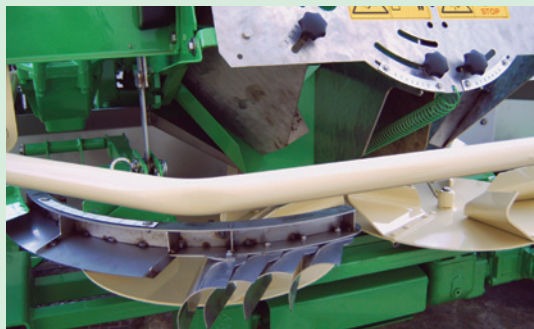
Border spreading with deflector II, switched - on.
