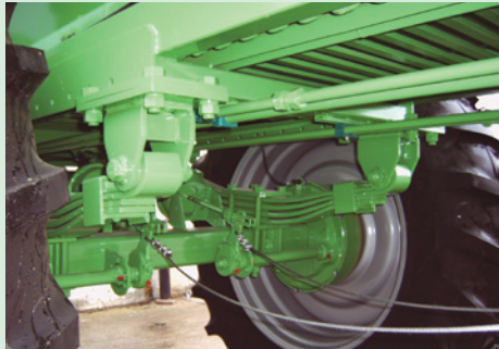
Spring suspension of axle.
