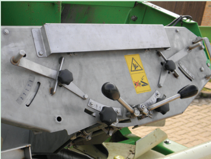
Guiding device for section control, automatic reduction of spreading width (option).
