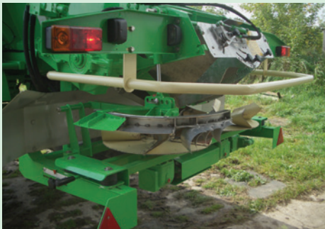
Hydraulically operated border control.
