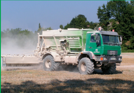
MAN with mounted spreader and 8 m - spreading screw.
