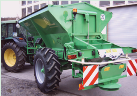
Single - disc system for winter road services (gritter).
