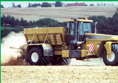
Mounted spreader on Terra Gator.
