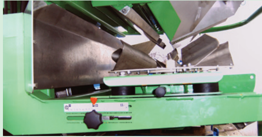
Spreading table „fore & aft“ adjustment without tools.
