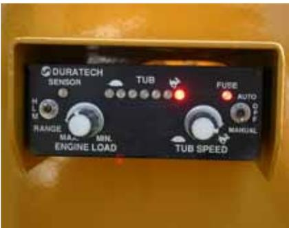
The DuraTech electronic governor slows protection for the tractor and the machine. This governor maintains a constant load on the tractor and driveline by adjusting the tubs rpm which controls the feed rate of the material to the hammermill.
