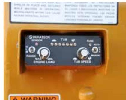
The tub rotation is controlled by an electronic governor that stabilizes engine load by adjusting the tub speed based on rotor speed. It also controls tub direction and tub stop.
