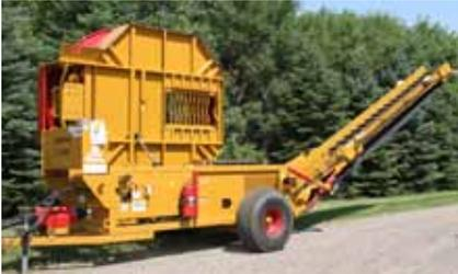
The H-1130's tub opens a full 90 degrees for easy access to the hammermill and drive train for service and maintenance.
