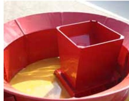
High-capacity grain grinding is another important operation that the H-1000 can also accomplish. By placing the optional grain-grinding hopper over the hammermill opening and changing screens, the H-1000 becomes a high capacity grain grinder for grinding and/or cracking feed grains.
