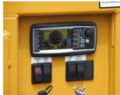
On the H-1030, the tub rotation feeds the hammermill using a Wachendorf Electronic Control Governor, which stabilizes engine load by adjusting or stopping the tub speed. It also controls tub direction, clockwise, stop, and counter-clockwise as well as tracking grinding hours.
