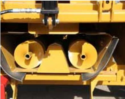
The dual 9" high-capacity augers mounted in the belly pan discharge the ground product to the stacking conveyor. The belly pan provides a clean area to catch and discharge small product such as ground corn and barley.
