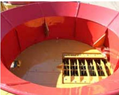
The H-1000 tub 10' 3" wide and 44 1/2" deep and is constructed of a 10-gauge steel floor and a 14-gauge steel side wall. The H-1000 tub has the capacity to handle all types and sizes of bales.
