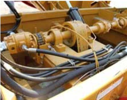
The 8 multiple belt drive system has been designed to handle increased horsepower and rotor speed. The spring tension belt drive system allows for constant belt tension while belts stretch and wear without having to manually adjust.
