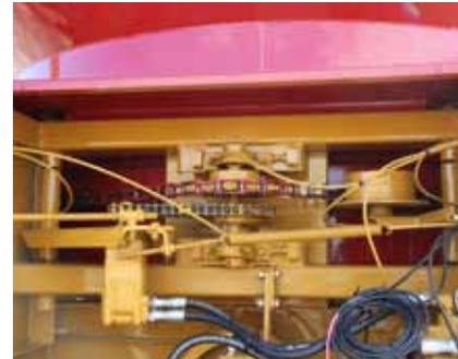
The H-1000 tub is driven by a hydraulic motor which drives a heavy-duty roller chain. The sprocket on the tub is a continuous sprocket that provides a positive and smooth transmission of power to the tub.
