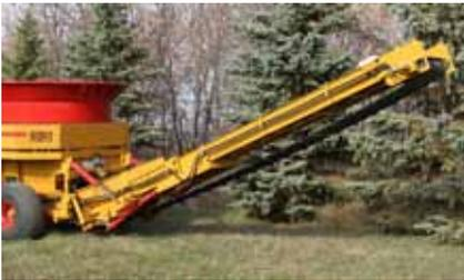
The 21' long x 24" wide hydraulically-folding conveyor is designed for the increased capacity of a 10' tub grinder. The conveyor folds over the top of the tub for easy transport. It is capable of stacking material up to 14' 9" high at a the maximum angle.
