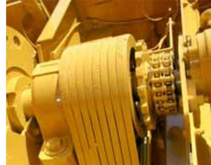
The belt drive system for the hammermill has 8-5 VP belts to handle the increased rotor speed and increased horsepower capacity. The spring tension belt drive automatically adjusts belt tension as the belts stretch.
