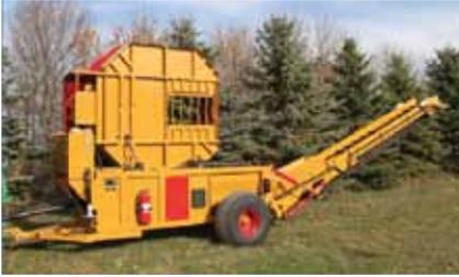
The H-1030's tub opens a full 90 degrees for easy access to the hammermill and drive train for maintenance and service.
