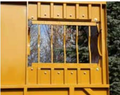
The heavy-duty bolt-in mill grate/slug bar combination is designed to allow the operator the ability to change the number of mill grate bars and slug bars as grinding conditions change. A geyser plate can be added to prevent product from being tossed straight up and out of the tub.
