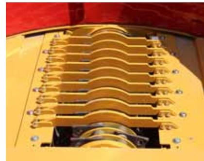
The new heavy-duty bolt-in mill grate/9 bar mill grate combination is designed to allow the operator the ability to change the number of mill grate bars and slug bars as grinding conditions change.
