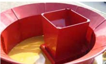
High-capacity grain grinding can also be done with the H-1130 tub grinder. Just add in the grain hopper and change the screens and you have a high capacity grain grinder for grinding and/or cracking feed grains.
