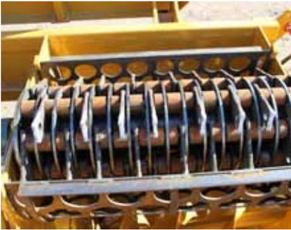
The H-1030 is equipped with a 44" long heavy duty hammermill that has been positioned to the rear of the tub. With the mill in the back, the ground product can quickly be discharged and transferred to the stacking conveyor. The hammermill is constructed of 3/8" thick plates with 1 1/4" case-hardened rods that hold 64-3/8" hammers. These hammers can be rotated and flipped for many hours of grinding. The mill is mounted to the frame with two 3" pillow block bearings on a 3 1/2" stress-proof shaft.
