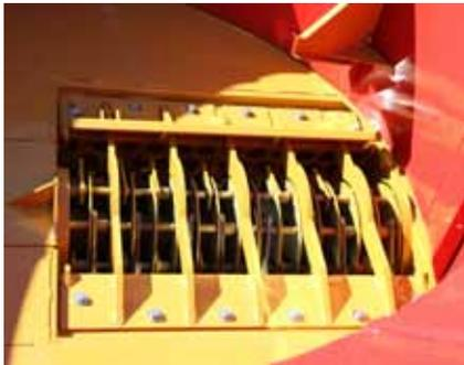
The hammermill is constructed of 3/16" thick x 15 3/4" diameter plates with 15/16" case hardened rods that hold 64-3/8" hammers. These hammers can be rotated and flipped for many hours of grinding.
