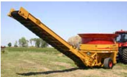
The hydraulic folding 24" wide by 26' long high-capacity stacking conveyor is designed for the increased capacity of the H-1130. It can stack material 18' 6" high.
