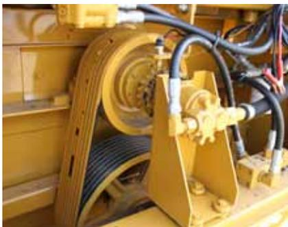
The 8-groove belt system delivers sufficient power from the PTO to the hammermill. The system has a fixed belt tension to accommodate, stretch and wear without having to monitor belt tension. This drive system turns the mill at approximately 2 x PTO speed. This mill speed provides for smooth feeding and delivers high capacity grinding performance.
