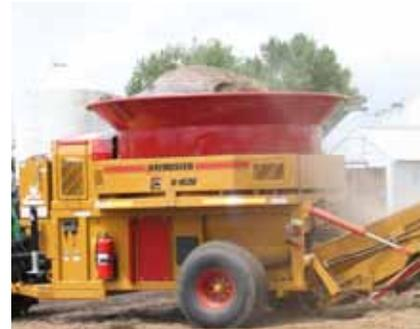
The H-1030 has a 10' 3" wide heavy-duty tub. The tub is 44 1/2" deep and will handle all types and sizes of bales.
