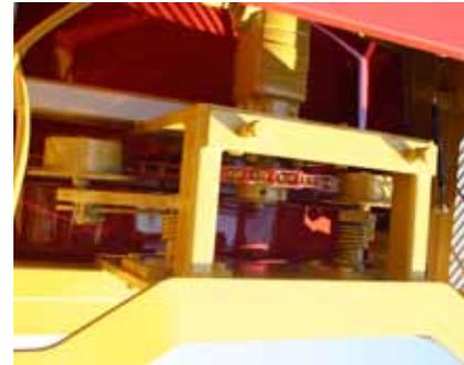
The tub drive has continuous teeth around the tub and dual spring tensioners. Power is provided by a single hydraulic motor controlled by the electronic governor.
